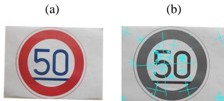
Figure 2. (a) Image of landmark; (b) Sift features found with scale and orientation
