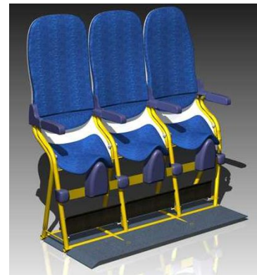
Figure 2. SkyRider Vertical Seat Design Concept [9]
